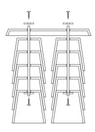
**06**. Insert the washers on top, cut off any excess wood and tighten all the screws until stable
