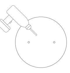
**02**. Using a drill bit for ceramics or tiles, make two holes in <u>one</u> of the pot plant plates
