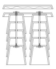
**08.** Place on top to cover the screws and add a weight for the entire drying time of the glue
