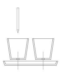
**01**. Use the holes in the pot plants to mark where to drill the holes in <u>one</u> of the pot plant plates
